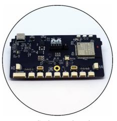
The control board also speaks to Marty's motors and sensors to find out what they are reading. Again, this is similar to our own nervous system, which receives signals from our senses. You can use Marty's brain to send signals to the servo motors and read sensors (like obstacle or position sensors) to allow Marty to physically react when sensing something – like shaking hands if there is a force on the arm.
